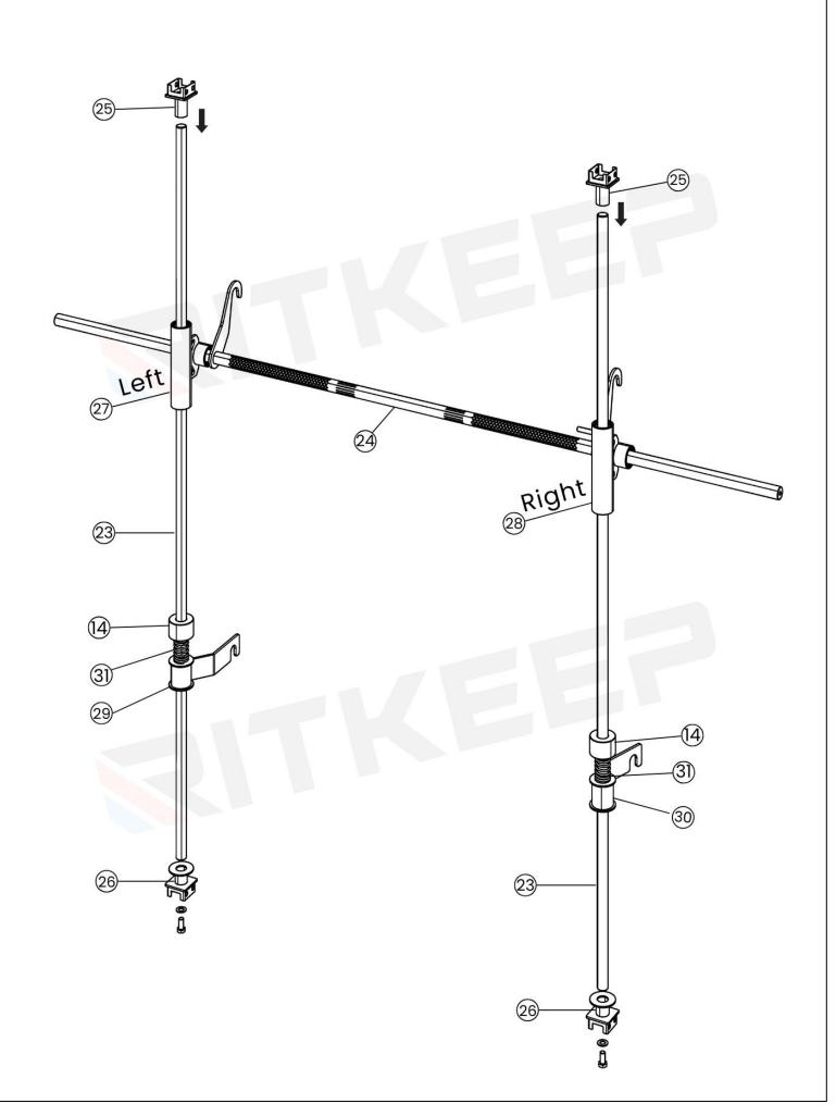
STEP 8 Do not tighten all bolts until all installations are complete.
