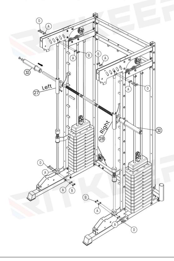
STEP 9 Do not tighten all bolts until all installations are complete.
